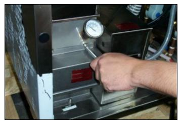
Removing the heater cover.
